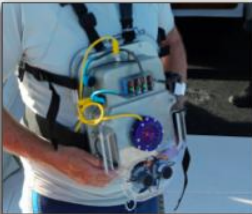
Figure 7. CHAT – Underwater wearable computer with real-time sound recognition used in the Bahamas with free-ranging Atlantic spotted dolphins. Picture used with permission – Wild Dolphin Project.
